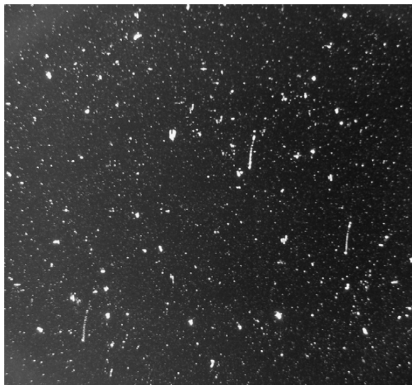
Figure 5.16 A photograph of pinholes in a 30 mm \times 30 mm sample of metallized film simply held up in front of a table lamp. This is a severely damaged surface. A photograph of pinholes for a better quality film is shown in Chapter 8 (Fig. 8.13).
