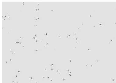
After cleaning – Particle count = 87
