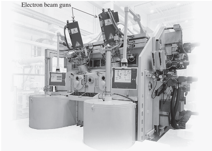
Figure 15.2 A 2.5 m wide twin electron beam evaporation system showing the two electron guns angled down and in to the source crucible. Photograph courtesy of Applied Materials
