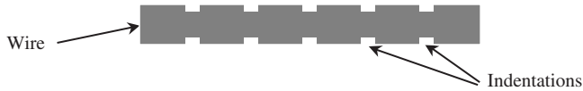
Figure 16.13 A schematic showing the indentations that may be caused by knurled drive wheels leading to aluminum pool fluctuations.
