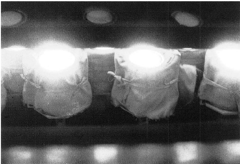
Figure 17.5 A photograph from a ULVAC vacuum coater that shows some induction-heated sources in action. The induction coils are hidden from view by the heat-insulating fabric wrapped around each source.
