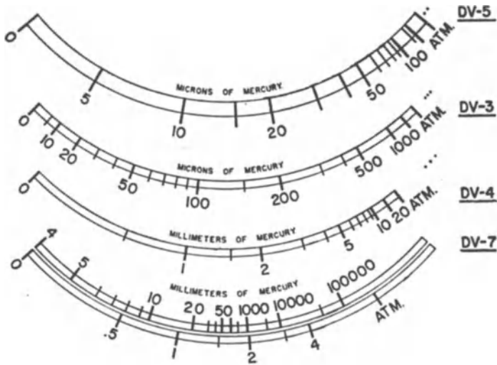
Figure 2.22 Calibration scale shapes for the four gauges designed by Benson 37 .
