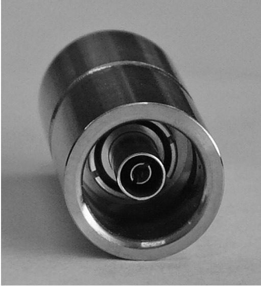
Figure 17.43 Triaxial feedthrough for the measurement of very low currents.
