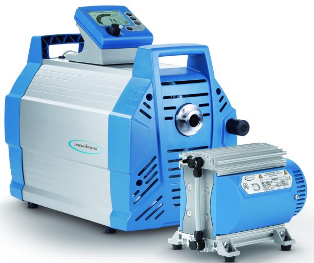
Figure 7.6 Two diaphragm pumps by VACUUBRAND: (a) MV 10 NT VARIO: 12.1 \text{ m}^3 \text{ h}^{-1} , 30 Pa; (b) MD 1 VARIO-SP: 1.8 \text{ m}^3 \text{ h}^{-1} , 100 Pa (compare Table 7.2).
