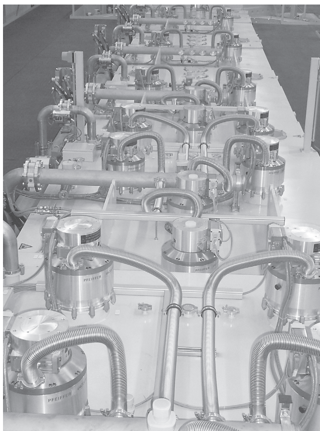
Figure 10.28 Aluminum foil coating system for high light reflection with TPH 2301 turbomolecular pumps. In this so-called air-to-air system, the aluminum foil is supplied into the continuous coating process system from air
