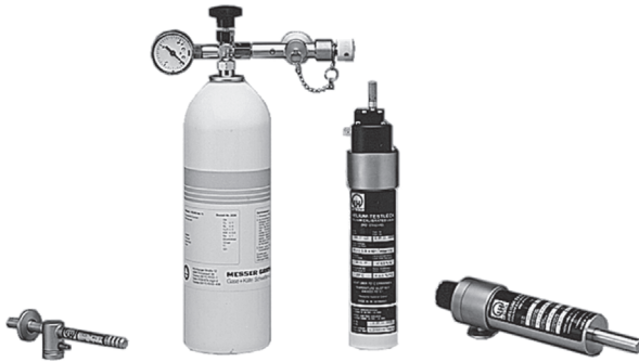
Figure 14.37 Selected test leak designs. From left to right: capillary-type leak (range > 10^{-4} \text{Pa } \ell \text{s}^{-1} ) without reservoir; capillary-type leak with manual valve, test gas reservoir, and adjustable upstream pressure for leakage rates from 10^{-4} to 10^{-2} \text{Pa } \ell \text{s}^{-1} ; built-in test leak with solenoid valve (permeation or capillary type); permeation-type test leak (range < 10^{-6} \text{Pa } \ell \text{s}^{-1} ) with manual valve and helium reservoir.
