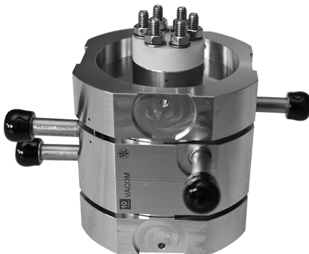
Figure 17.41 Resonant beam position monitor with electrical feedthrough.
