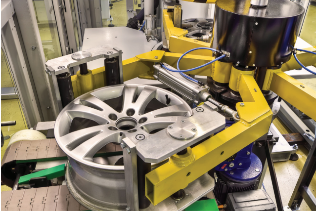
Figure 19.14 Fully automated test system for aluminum wheels (Von der Heyde, Stade, Germany). Apart from actual measurement, the system also performs the operations “load/unload,” “sort,” “label.” Main technical specifications: leak rate: 10^{-4} mbar \ell s^{-1} ( 10^{-2} Pa \ell s^{-1} ) with automatic calibration
