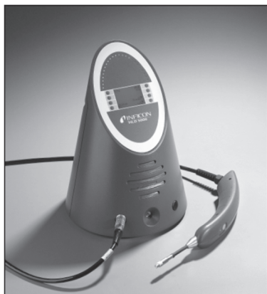
Figure 14.38 Sniffer leak detector for refrigerants operating on infrared absorption (the complete detection system is integrated into the sniffer handle).
