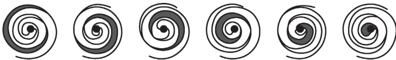
Figure 7.36 Gas path in a scroll spiral. Courtesy of E. Reuschling, Edwards GmbH .
