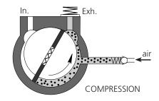
the partial pressure of the pumped gas is less than its saturated vapour pressure at the temperature of the pump. Condensation is therefore impossible if this limit is not reached. The maximum admissible vapour pressure is obtained at the pump inlet for this value.
