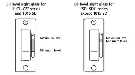
**Note:** Optimum pump performance and service life are obtained when the oil level is between the maximum level and the minimum level
