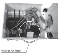
The voltage range can be read beside the motor switch: the dual frequency single-phase motor can be configured for low voltage (LV) or high voltage (HV).
