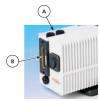
At the first start-up, to facilitate lubrication of the pump, pour a few drops of oil (1 to 2 cm³) through the inlet orifice.
